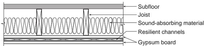
**Figure 3.** Resilient metal channels between two layers of 15.9-mm fire-rated gypsum board in the ceiling give this construction an STC of only 38. As shown in Table 4, removing the internal layer of gypsum board gives an STC of 52 for an OSB subfloor. Putting both layers below the resilient metal channels gives an STC of 55.
