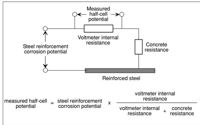
Figure 2. Schematic illustrating the half-cell measurement circuit
