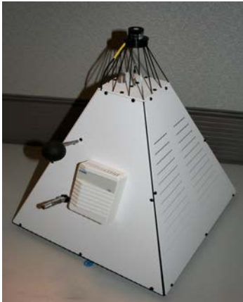
Figure 2: Indoor weather station
