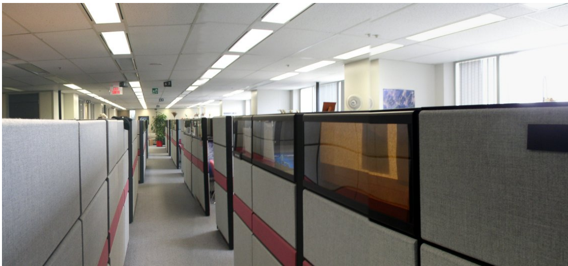
Caption. Is this the perfect panel design? With windows to the right, the use of transparent panels makes the panel low enough for daylighting purposes and also high enough for speech privacy. However, after installation these transparent panels are often covered by posters or coats by occupants seeking visual privacy. Note that to really improve daylight penetration into the second row of workstations from the window, the upper panels of the panels to the left should also be transparent.
