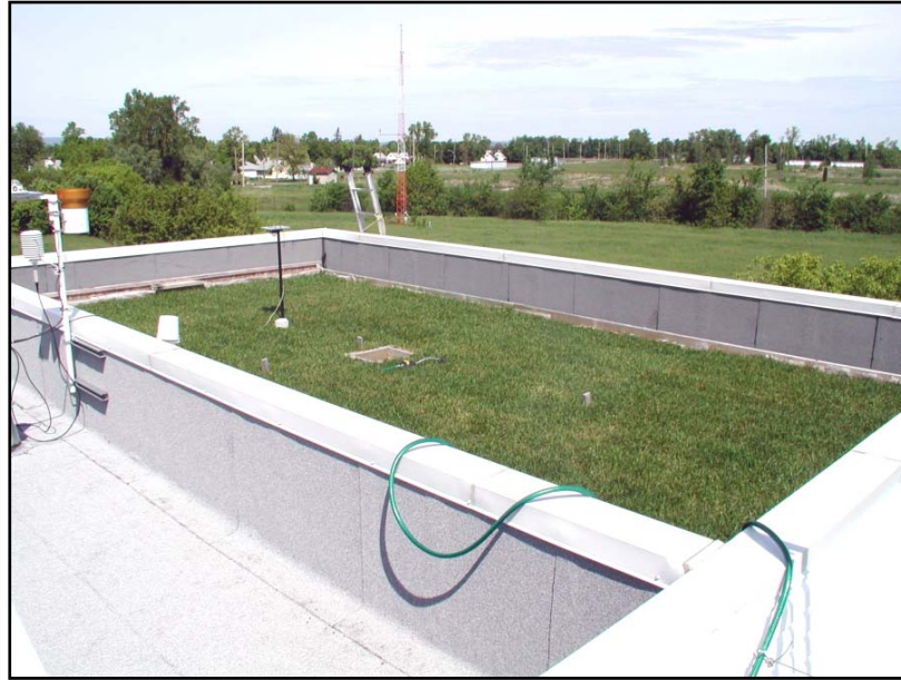
Figure 1: The sod two weeks after installing on the FRF in the NRC campus in Ottawa (2002). Note that the median divider separates the Green Roof (left) and the Reference Roof (right). The weather station is located at the median divider.
